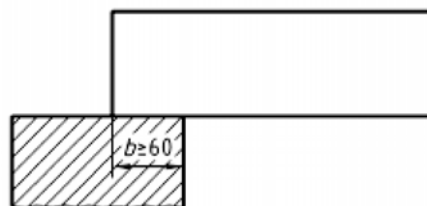
b) beams without protruding reinforcement
