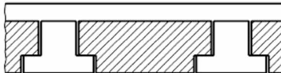
Figure B.4 — Floors with self-bearing beams
