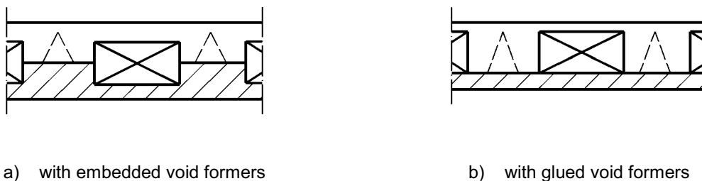
Figure B.2 — Examples of hollow composite slabs
